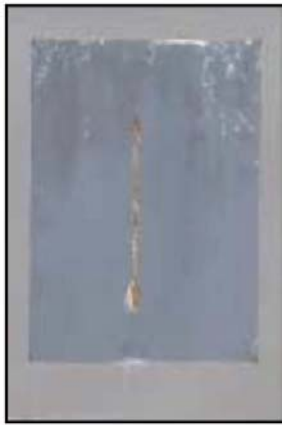
Salt spray resistance 耐盐雾, 2000h DFT干膜厚度: ~50um BECKOPOX™ EP2390w/75MP- BECKOCURE™ VEH2849w/80WA
