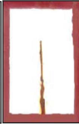
Salt spray resistance 耐盐雾, 2500h DFT干膜厚度: ~200um Layers层数: 3
